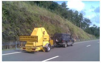
Figure 5-1: Falling Weight Deflectometer (FWD) machine
