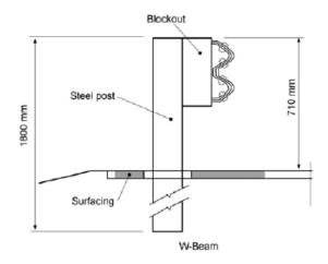
Figure 6-12: W beam barrier system
