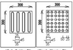
"Go" - Guiding Tile "Stop" - Warning Tile Figure 6-11: Tactile paving
