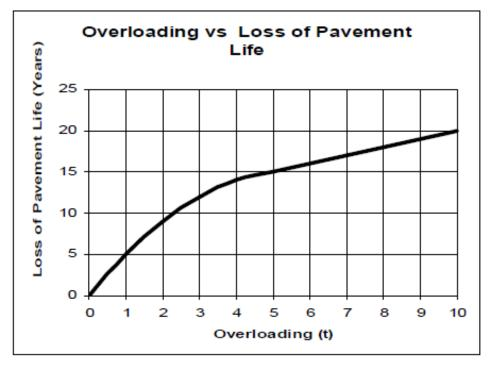
Figure 2-6: Loss of Pavement Life with Overloading
