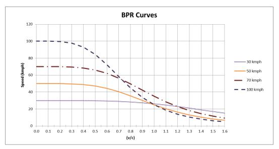
Figure 5-4: BPR Curve by Road Classification & Design Speed
