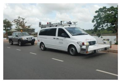
Figure 5-2: Multi-Function Network Survey Vehicle (MFNSV)
